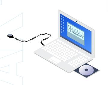
The logger can be read with a *PC*, a *Laptop*, using the **KOOLTRAK™** *Interface cable and software*. To collect data "touch" the cable to the logger. After a few seconds an audible and visual message confirms the data transfer.
